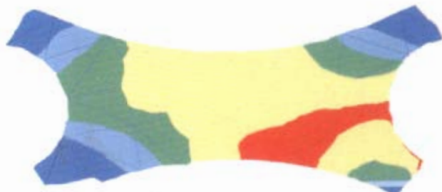
FEM Analysis of Membrane ensures minimum stress areas
