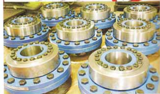
Large mecaloc shrink disc couplings for power generation.
