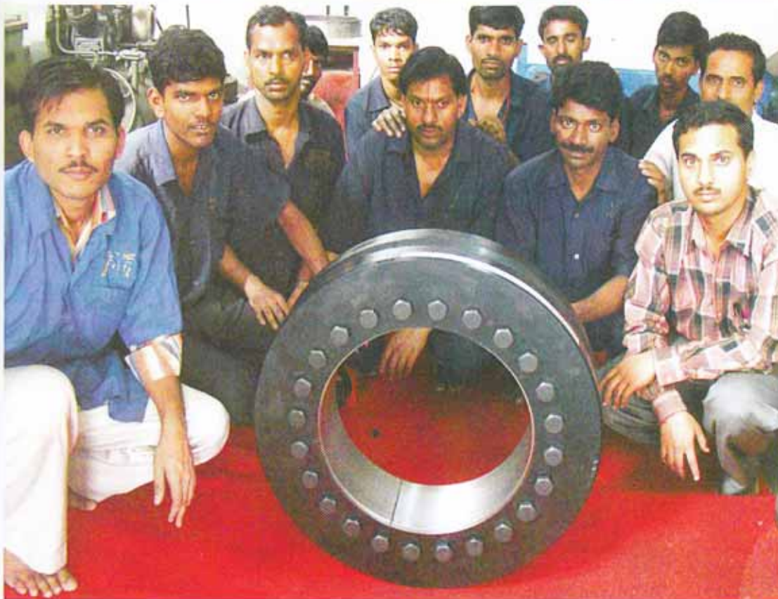
Mecashrinc shrink disc for shaft dia 420 transmitting 900,000 Nm torque on a briquetting press in a steel plant.
